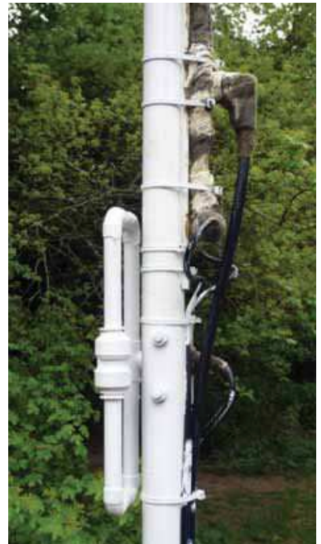
PHOTO 5: A completed dipole mounted on the pole with part of the power splitter on the right.
