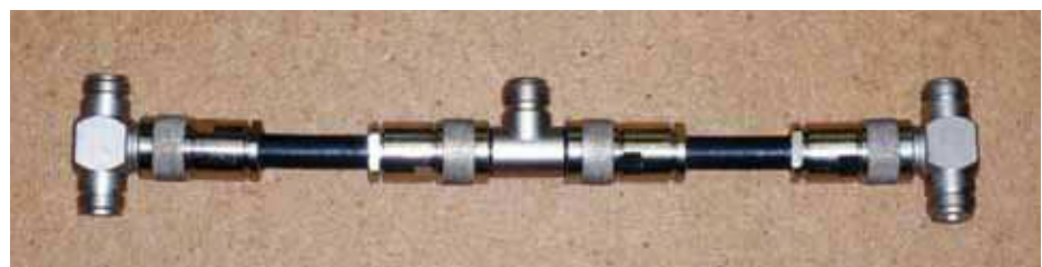
PHOTO 3: The 4-way power splitter.
