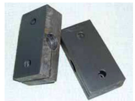
PHOTO 2: Two of the plastic blocks fabricated to insulate the dipoles from the support pole.
