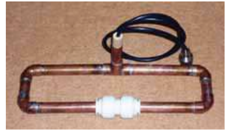
PHOTO 4: One completed dipole with feed cable.
